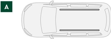
This is two separate longitudinal rails. An additional roof rack is necessary in order to mount the tent. Roof racks are vehicle-specific parts and must therefore always be matched precisely to the vehicle. Help in selecting the right roof rack is available from automotive accessories dealers or from a local vehicle dealer.
