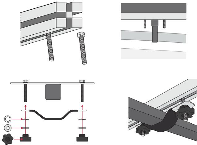
5. Tighten the screws of each fixed point in turn, then cover the guide rail cover in turn, and finally check the fixing status of each fixed point again. Installation is complete when there are no irregularities. Caution: Please pay attention to the order of gasket placement: flat washer- spring washer - plum knob nut.
