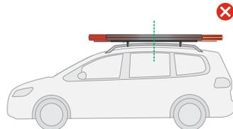
Screw the roof tent to the roof rack using the fastening system included in the scope of delivery. The roof tent is mounted to the roof rack with four fastening sets.
